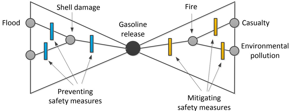
**Figure 2.** The bow-tie concept for a gasoline storage tank subject to natural disasters.
