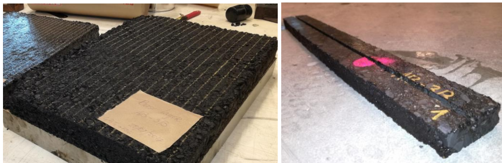
FIGURE 4 Prefabricated asphalt specimens with groove for FBGs embedment preparation
