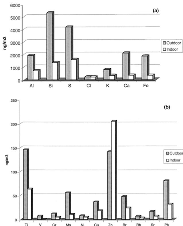
Fig. 2 Comparison of the outdoor and indoor elemental aerosol concentrations.
