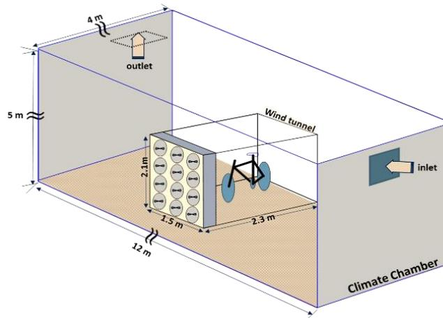
Figure 1. Schematic representation showing the used training bicycle fixed inside a customized wind tunnel and placed within the climate chamber.
