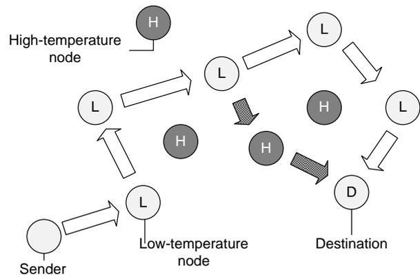
**Fig. 6** An example of LTR and ALTR. The white arrows indicate the LTR-path. The shaded arrows show the adapted path of ALTR. When the path has three hops, the routing algorithm switches to shortest path routing.
