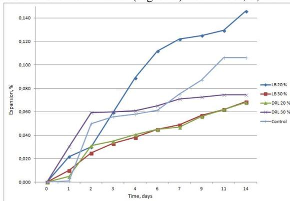
**Figure 3** ASR test results for DRL and LB
