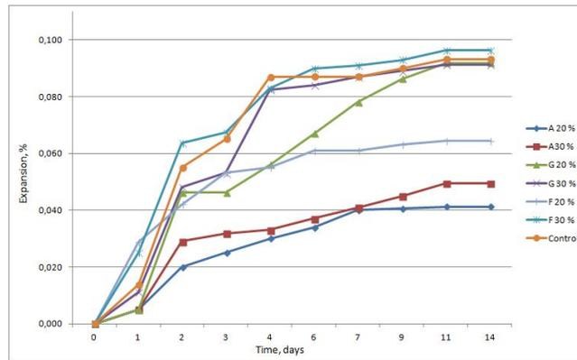
Figure 4 ASR test results for A, G and F
