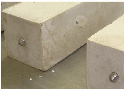
**Figure 2** ASR test concrete specimens with glass powder slurries
