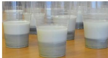
**Figure 1** Waste glass slurry samples
