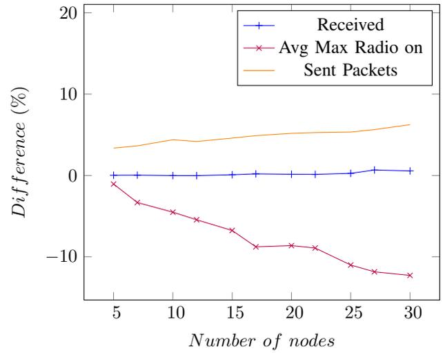
Fig. 16. Difference between whether or not overhearing was used. Data interval: 9.
