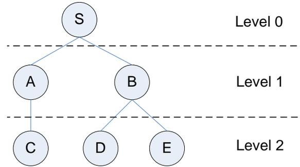
Fig. 1. Tree topology for a network of 5 nodes
