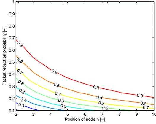
Fig. 10. Probability that node  $n$  is capable of hearing its parent's scheme or to do a full recovery, calculated with (9). The curves connect the points with the same probability. The x-axis is the position of node  $n$  in the control sub cycle, the y-axis is the packet reception probability. It can be seen that overhearing is useful.
