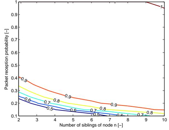
Fig. 11. Probability that node  $n$  is capable of hearing its parent's scheme or to do a full recovery, calculated with (12). The curves connect the points with the same probability. The x-axis is the number of siblings of node  $n$ , the y-axis is the packet reception probability. It can be seen that overhearing is useful when more nodes have the same parent.
